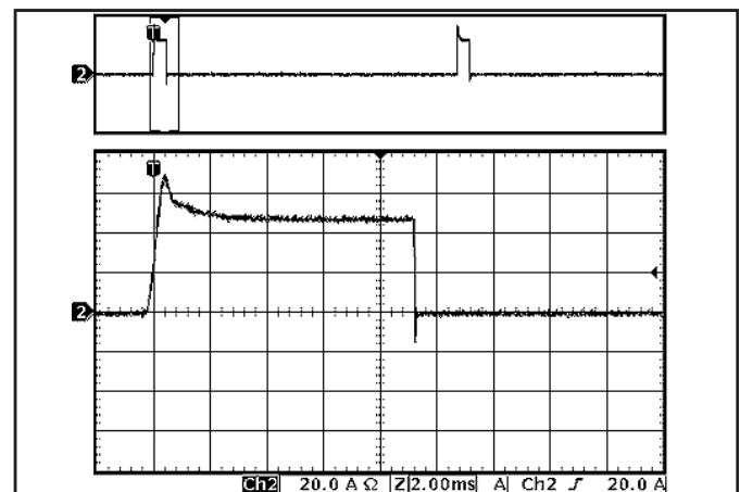
Figure 18: Load current (20A/div) as a function of time when the converter attempts to turn on into a 1\ \text{m}\Omega short circuit. Bottom trace (2ms/div) is an expansion of the on-time portion of the top trace.
